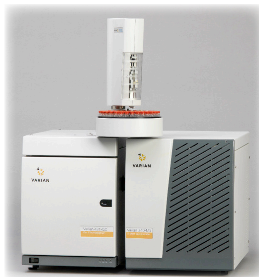
Figure 2. Varian 220-MS ion trap mass spectrometer with 431-GC gas chromatograph and 8400 AutoSampler.
